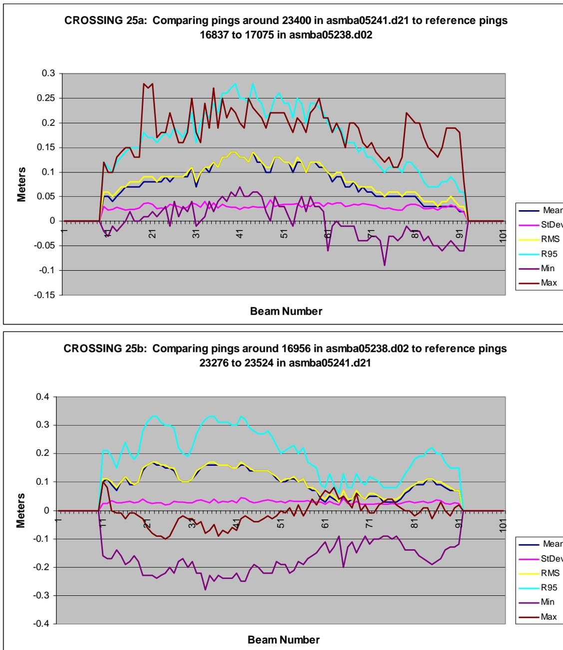
**Figure 3.1-3.** HARS Crossing 25a/b: Beam-to-beam comparison between the nadir beams (reference pings) and all beams for a cross lane and a main-scheme lane in an area of overlap. Top panel uses the cross lane as the reference and the bottom panel uses the main-scheme lane as the reference.
