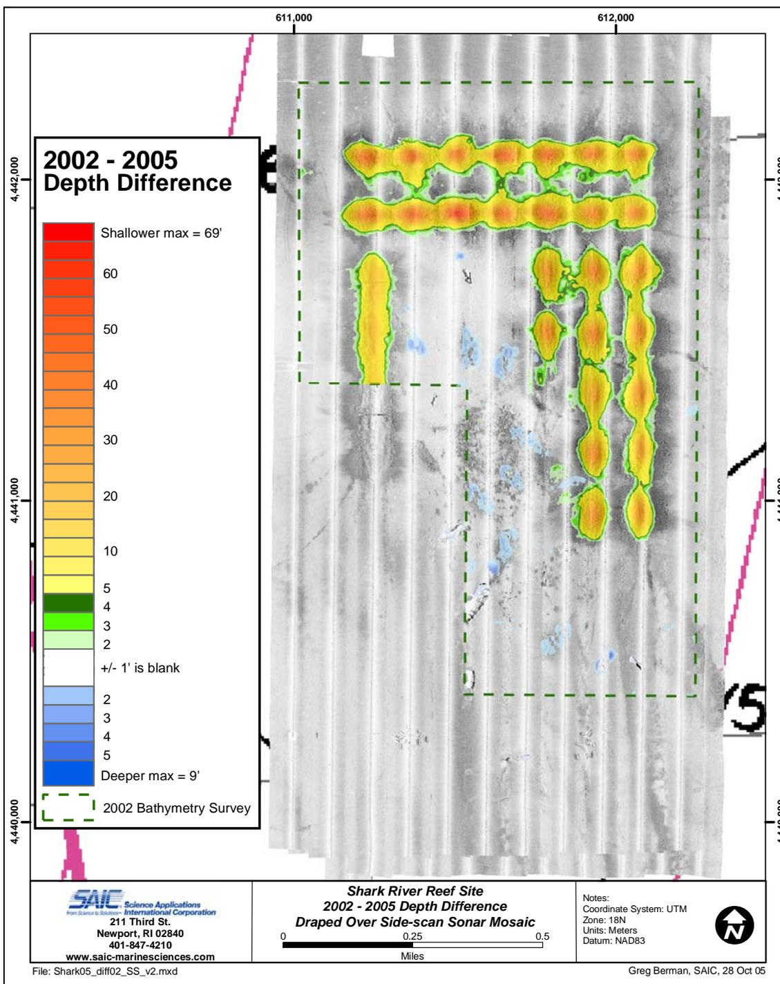
**Figure 3.3-5.** Bathymetric depth difference between the August 2005 multibeam survey and the January 2002 survey over the Shark River Reef
