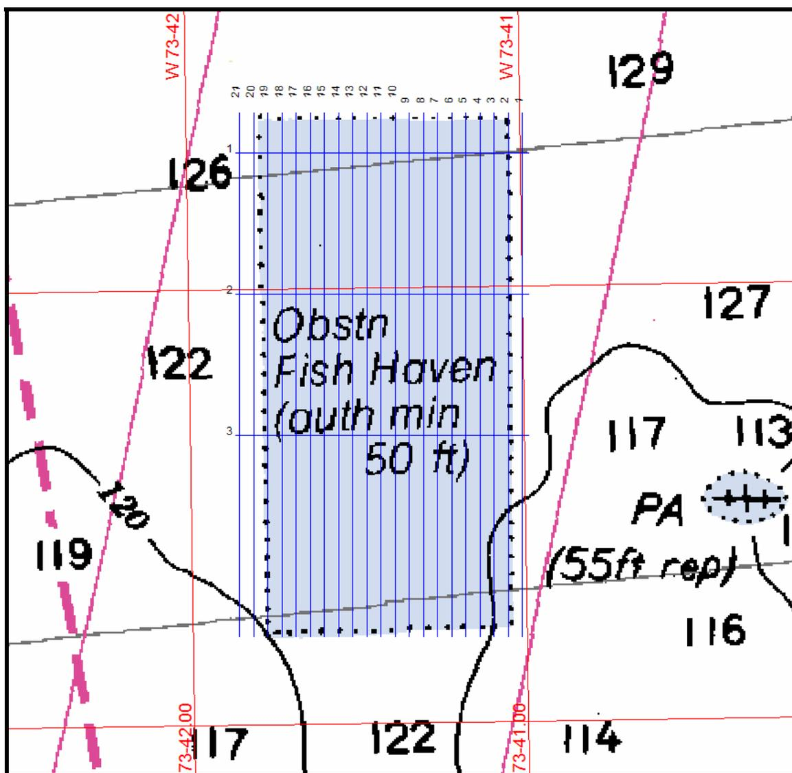
**Figure 2.1-3.** Depiction of north-south main scheme lanes (spaced at 60 and 30 m intervals) and east-west cross lanes that were occupied during the Summer 2005 multibeam survey operations conducted at Shark River Reef.
