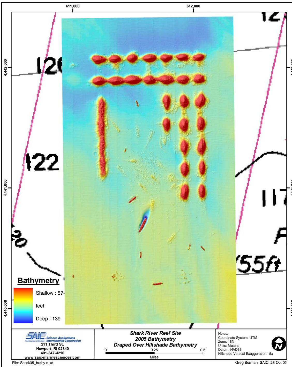
**Figure 3.3-1.** Hill-shaded gridded relief model based on the August 2005 bathymetric survey at the Shark River Reef
