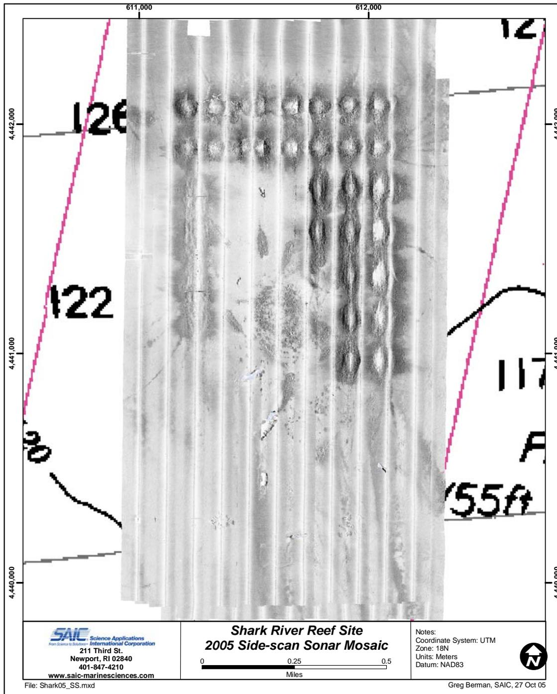
**Figure 3.3-2.** Side-scan sonar imagery mosaic based on the August 2005 bathymetric survey at the Shark River Reef
