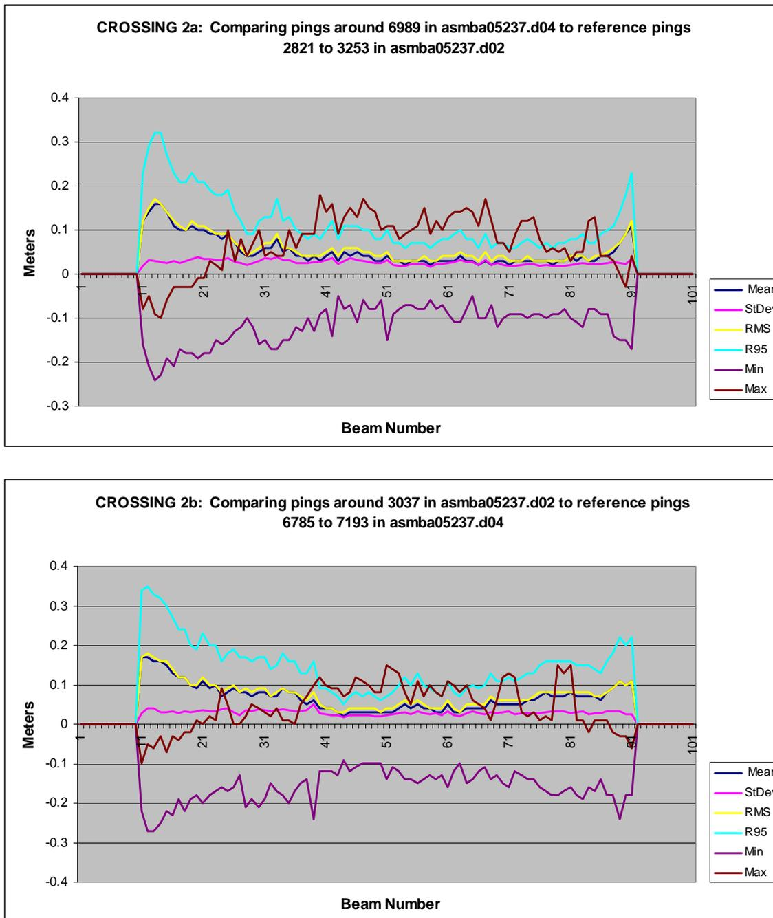
**Figure 3.1-5.** Shark River Reef Crossing 2a/b: Beam-to-beam comparison between the nadir beams (reference pings) and all beams for a cross lane and a main-scheme lane in an area of overlap. Top panel uses the cross lane as the reference and the bottom panel uses the main-scheme lane as the reference.
