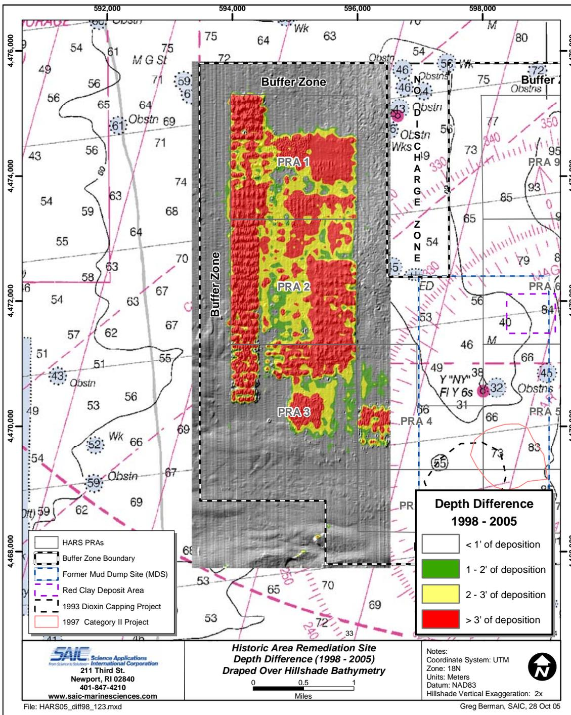
Figure 3.2-5. Bathymetric depth difference between the August 2005 multibeam survey and the September 1998 survey over PRAs 1, 2 and 3
