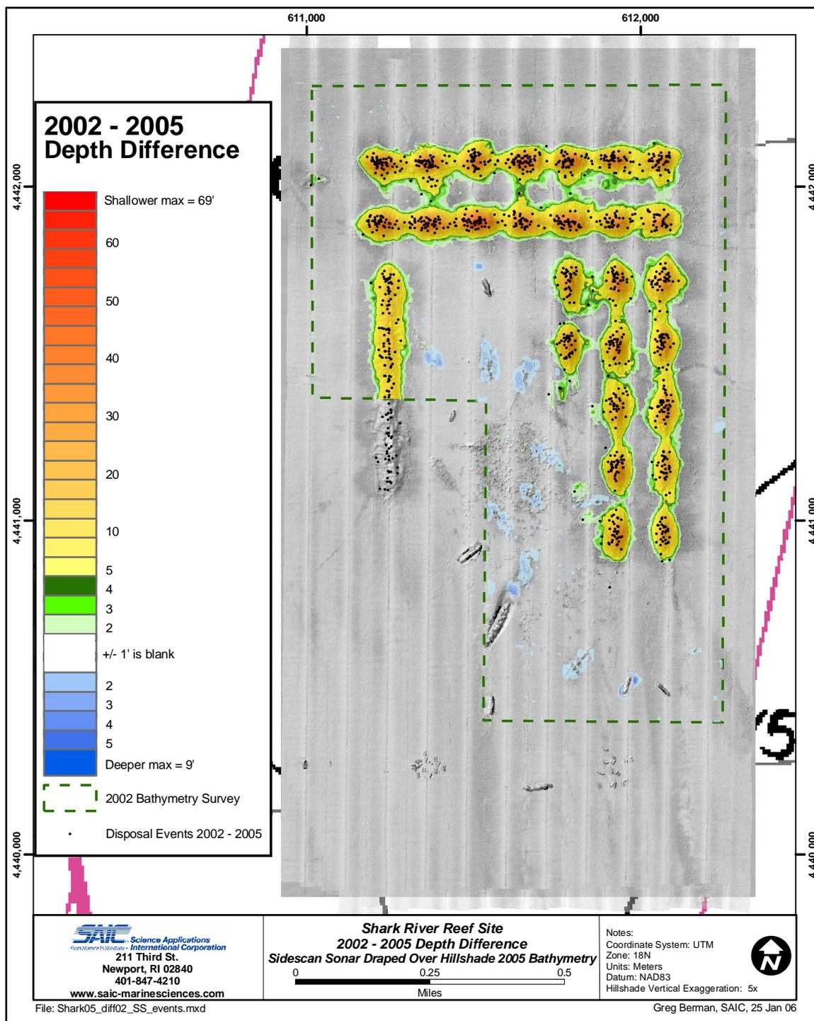
**Figure 3.3-6.** Disposal point data from the Shark River Reef from 2002 through 2005 depicted over the depth difference grid computed between the 2002 single-beam baseline survey and the 2005 multibeam survey; the 2005 side-scan sonar mosaic is included as the backdrop.
