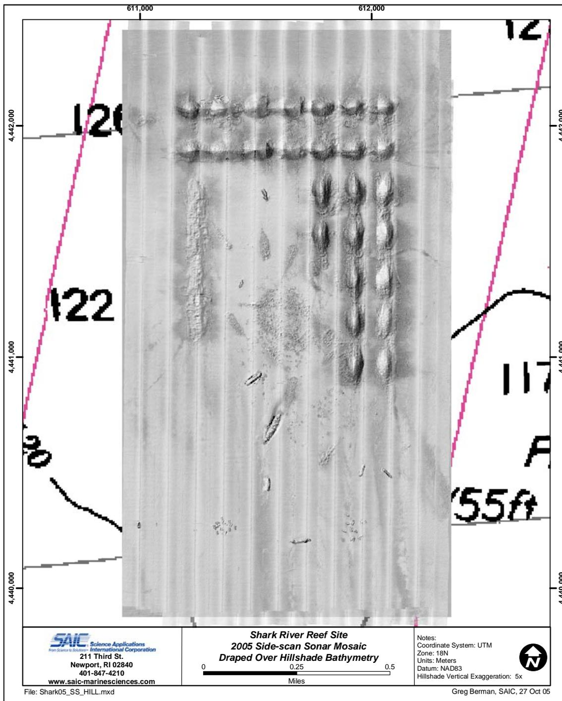
**Figure 3.3-3.** Multibeam backscatter imagery draped over the hill-shade multibeam bathymetry from the 2005 Shark River Reef dataset.
