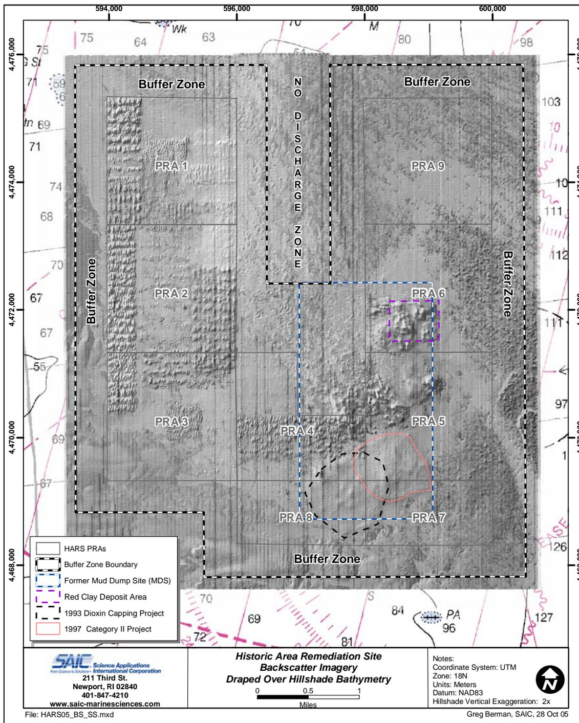
**Figure 3.2-3.** Multibeam backscatter imagery draped over the hill-shade multibeam bathymetry from the 2005 HARS dataset.
