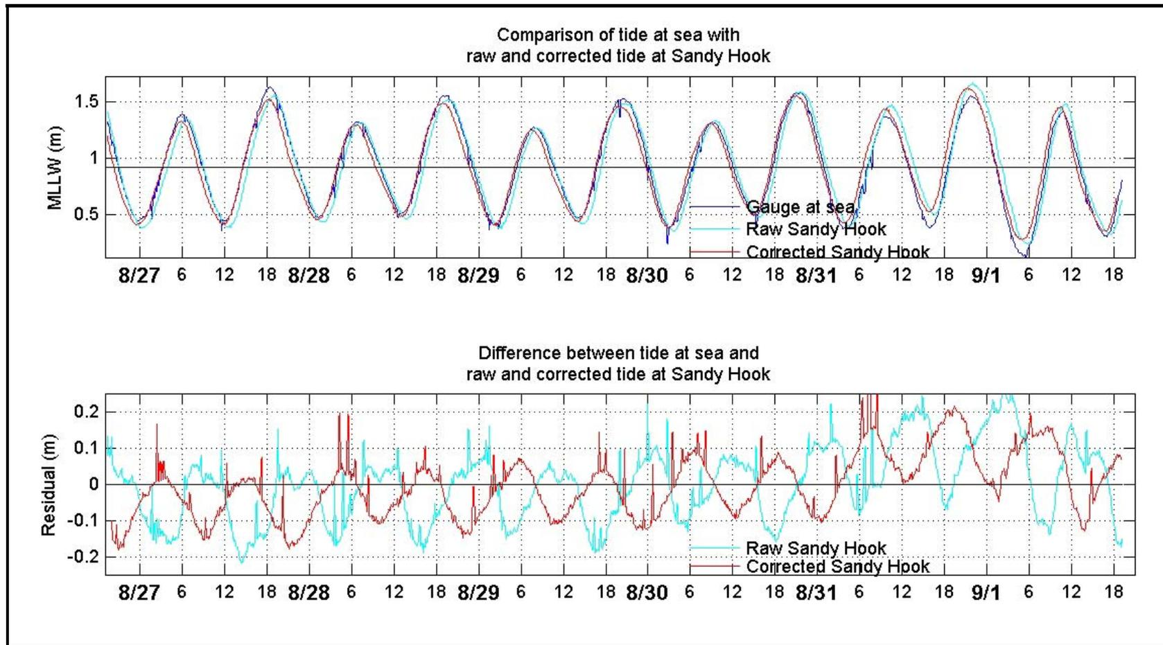
**Figure 3.1-1.** Time series comparison of the observed tidal heights from the NOAA Sandy Hook tide gauge (with and without offset correctors applied) and the HARS pressure tide gauge. Top panel provides time-series tidal heights relative to MLLW and the bottom panel provides the differences between the HARS pressure gauge and both the direct and offset Sandy Hook tidal values.
