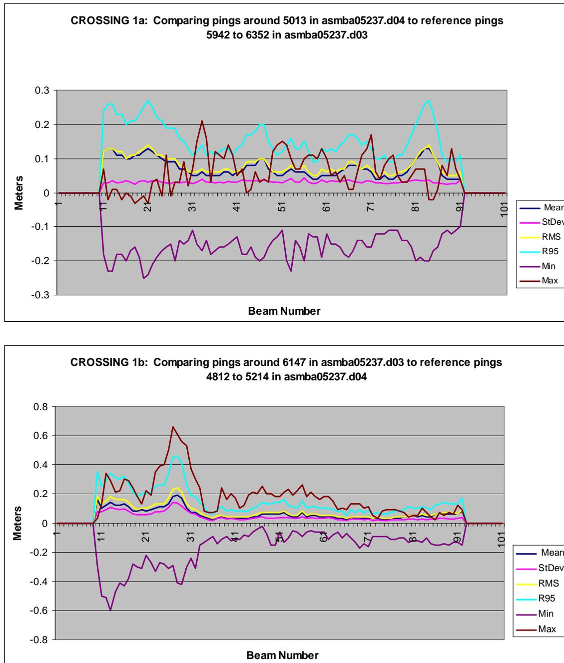
**Figure 3.1-4.** Shark River Reef Crossing 1a/b: Beam-to-beam comparison between the nadir beams (reference pings) and all beams for a cross lane and a main-scheme lane in an area of overlap. Top panel uses the cross lane as the reference and the bottom panel uses the main-scheme lane as the reference.
