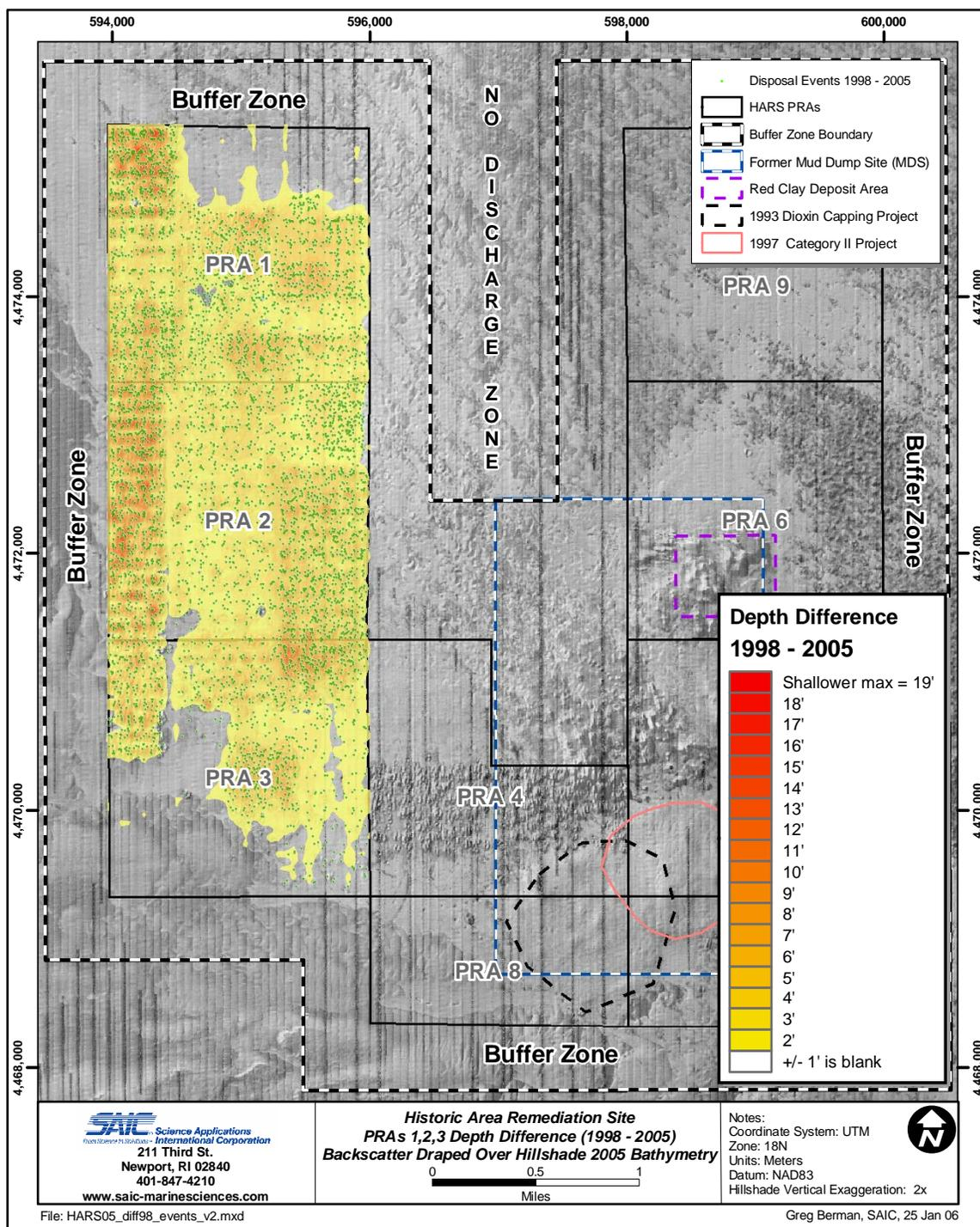
**Figure 3.2-6.** Disposal point data from the HARS from 1998 through 2005 depicted over the depth difference grid computed between a 1998 single-beam baseline survey of PRAs 1,2, and 3 and a 2005 multibeam survey of the entire HARS; the 2005 multibeam hillshade bathymetry and backscatter is included as the backdrop.
