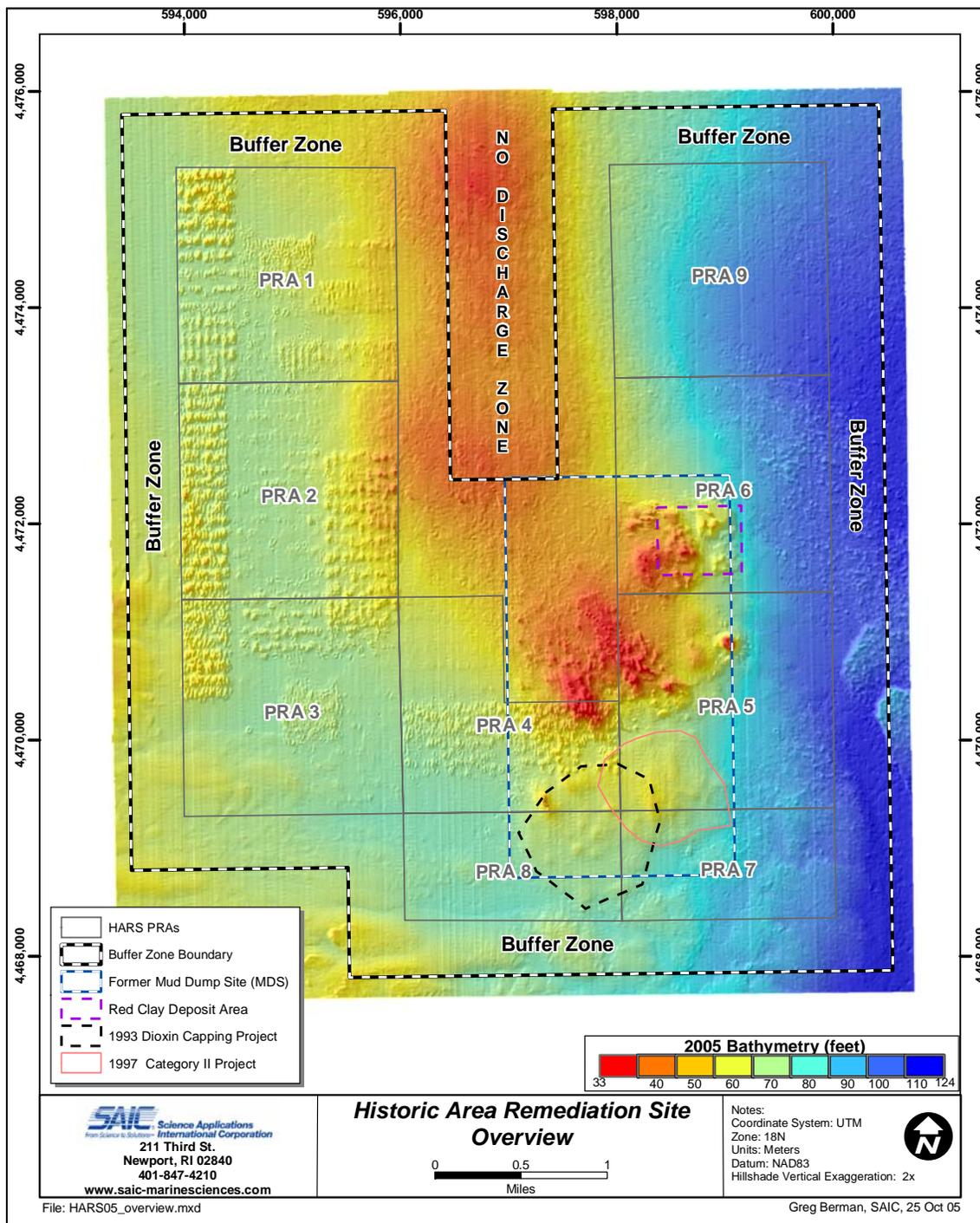
Figure 3.2-1. Hill-shaded relief model based on the August 2005 bathymetric survey at the HARS
