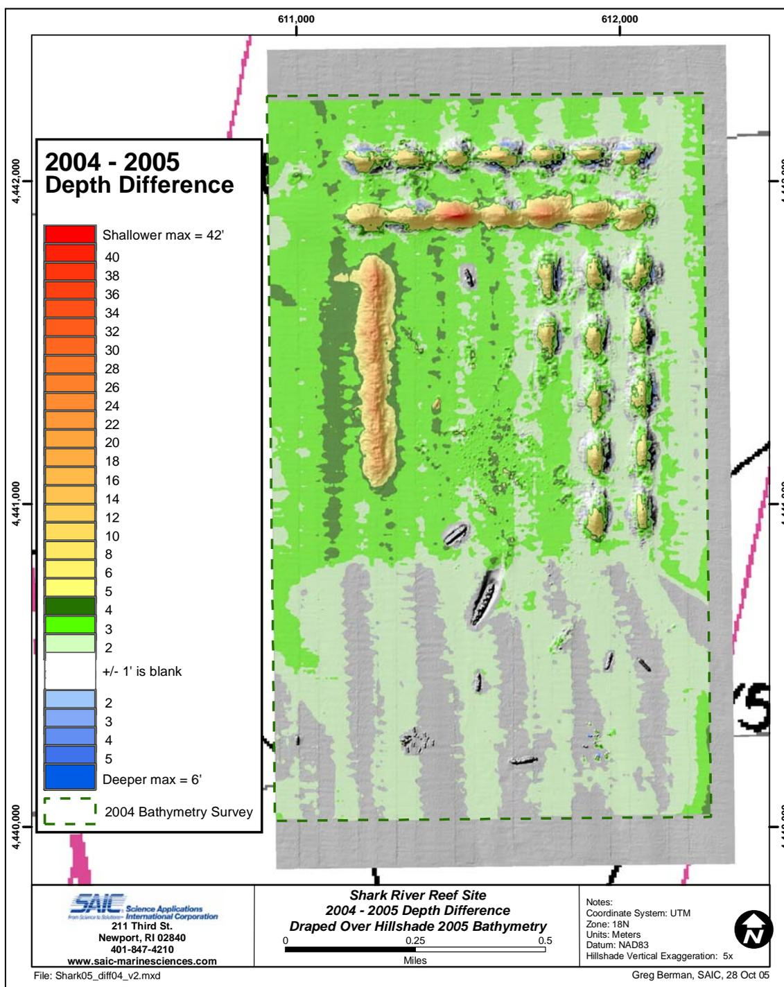
**Figure 3.3-7.** Bathymetric depth difference between the August 2005 survey and the May 2004 multibeam survey at the Shark River Reef
