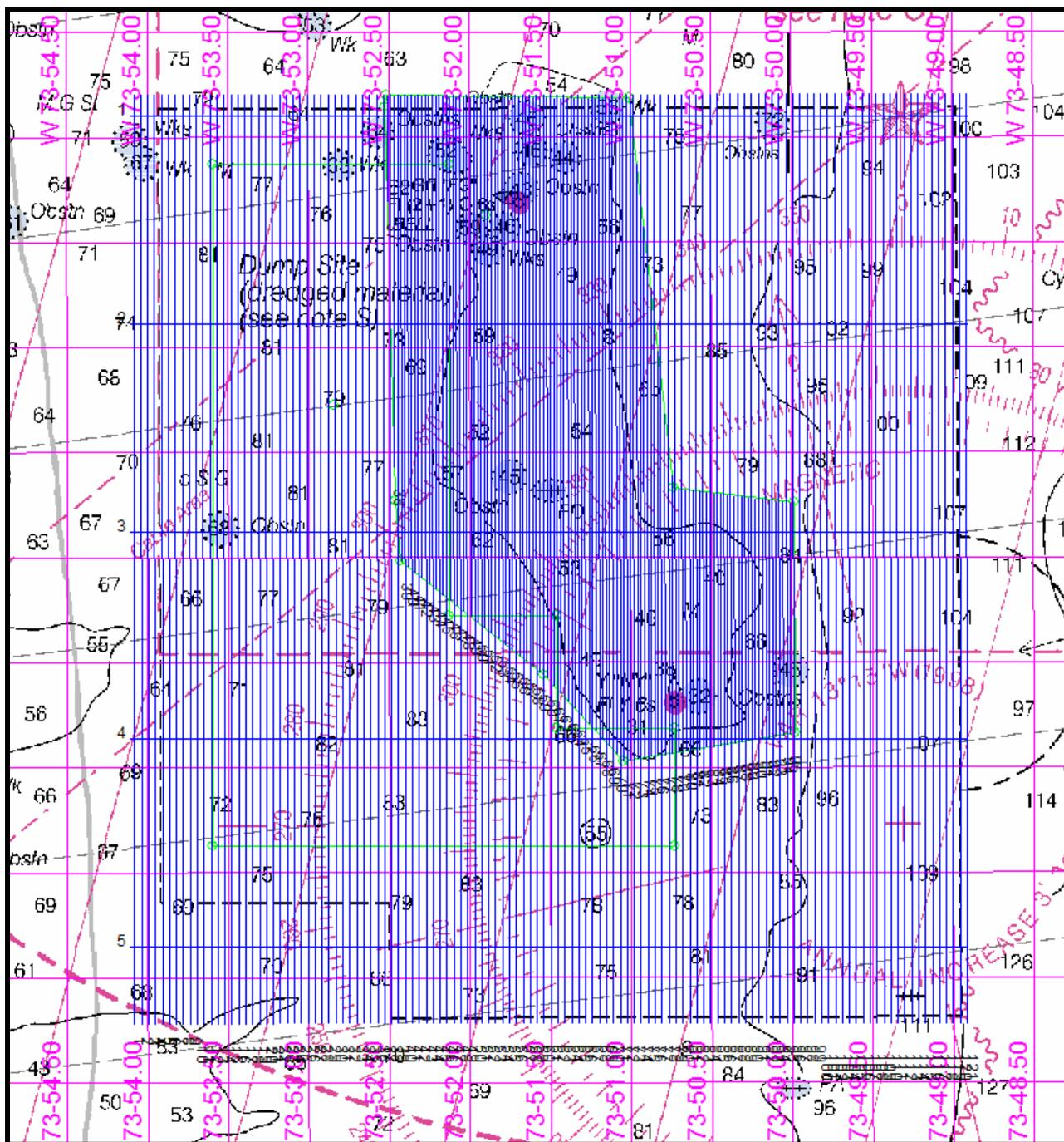
**Figure 2.1-2.** Depiction of north-south main scheme lanes (spaced at 60 and 30 m intervals) and east-west cross lanes that were occupied during the Summer 2005 multibeam survey operations conducted at the HARS.
