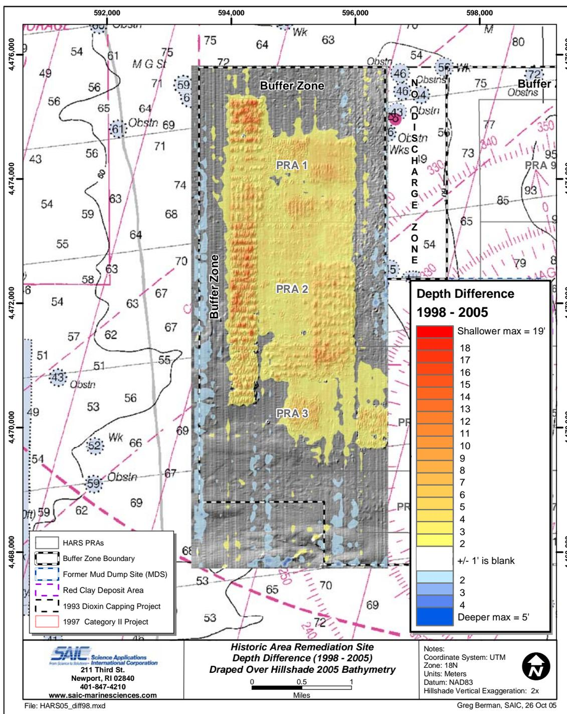
**Figure 3.2-4.** Bathymetric depth difference between the August 2005 multibeam survey and the September 1998 survey over PRAs 1, 2 and 3
