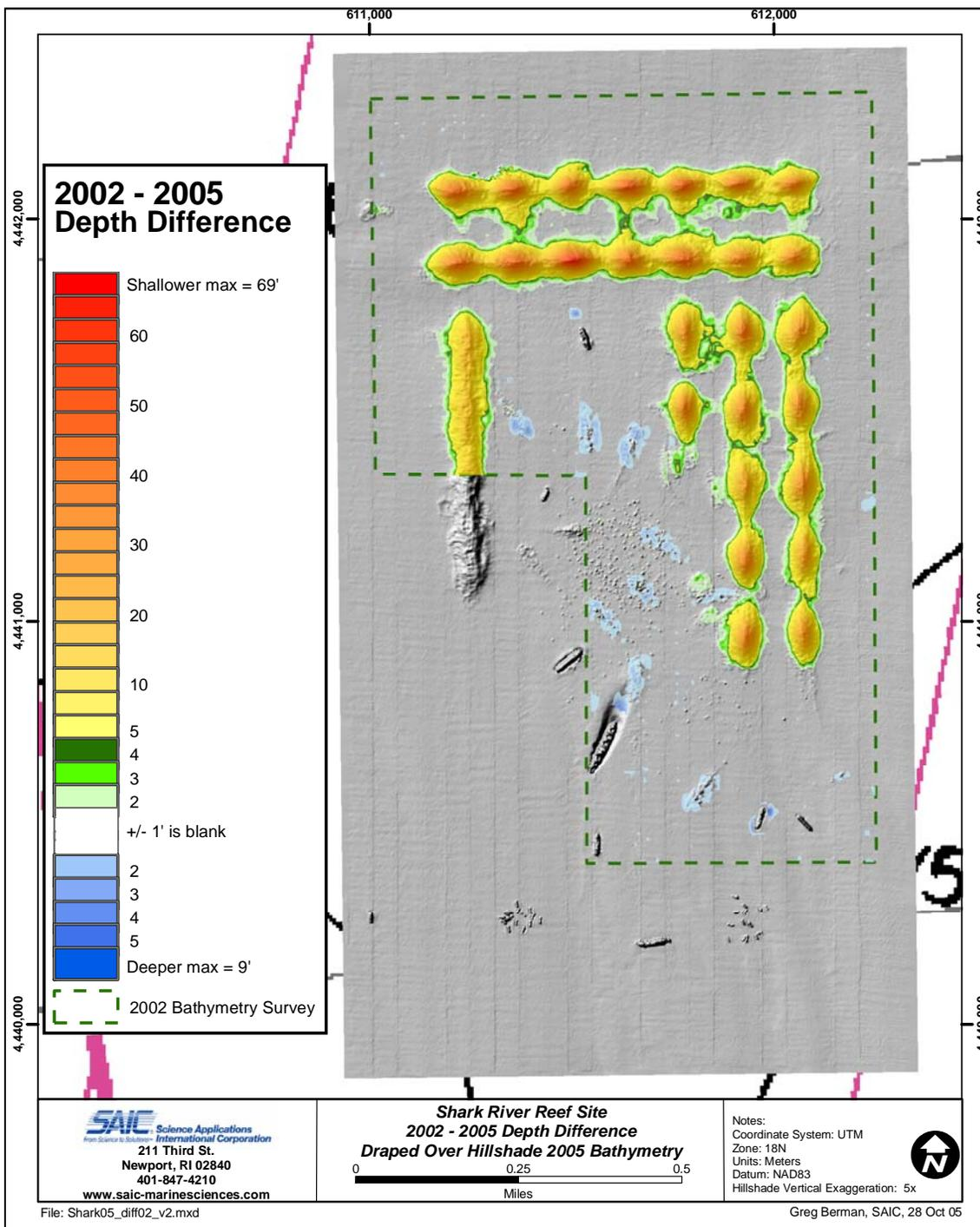
**Figure 3.3-4.** Bathymetric depth difference between the August 2005 multibeam survey and the January 2002 survey over the Shark River Reef
