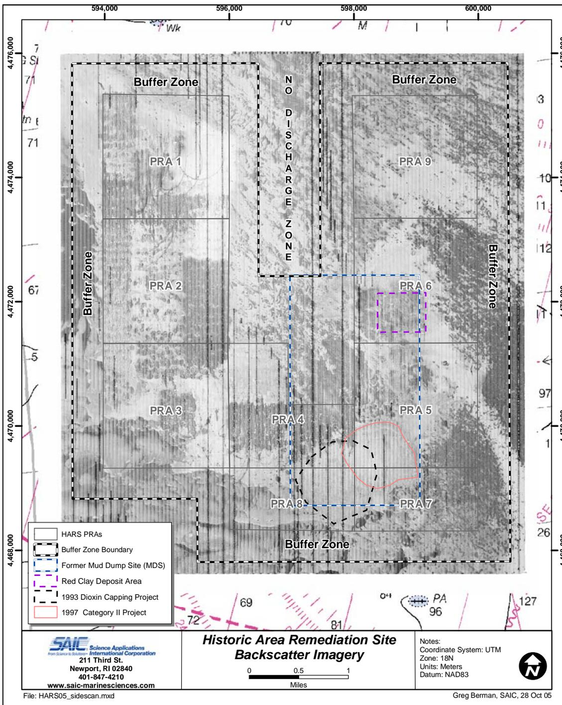
Figure 3.2-2. Multibeam backscatter imagery mosaic based on the August 2005 bathymetric survey at the HARS
