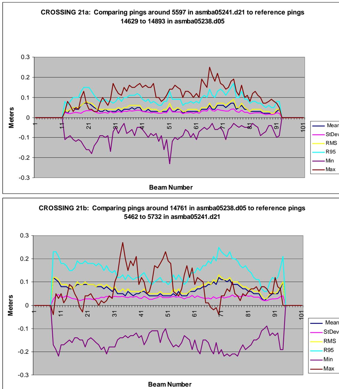
**Figure 3.1-2.** HARS Crossing 21a/b: Beam-to-beam comparison between the nadir beams (reference pings) and all beams for a cross lane and a main-scheme lane in an area of overlap. Top panel uses the cross lane as the reference and the bottom panel uses the main-scheme lane as the reference.
