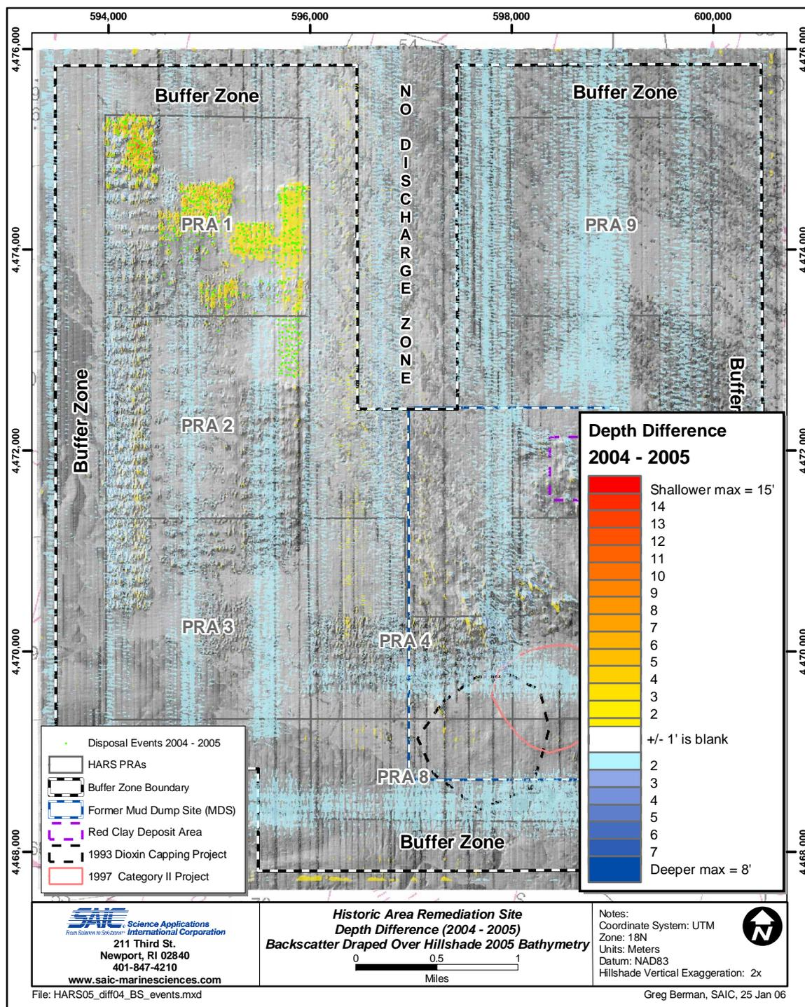
**Figure 3.2-8.** Disposal point data from the HARS from 2004 and 2005 depicted over the depth difference grid computed between multibeam surveys conducted in October 2004 and August 2005; the 2005 multibeam hillshade bathymetry and backscatter is included as the backdrop.
