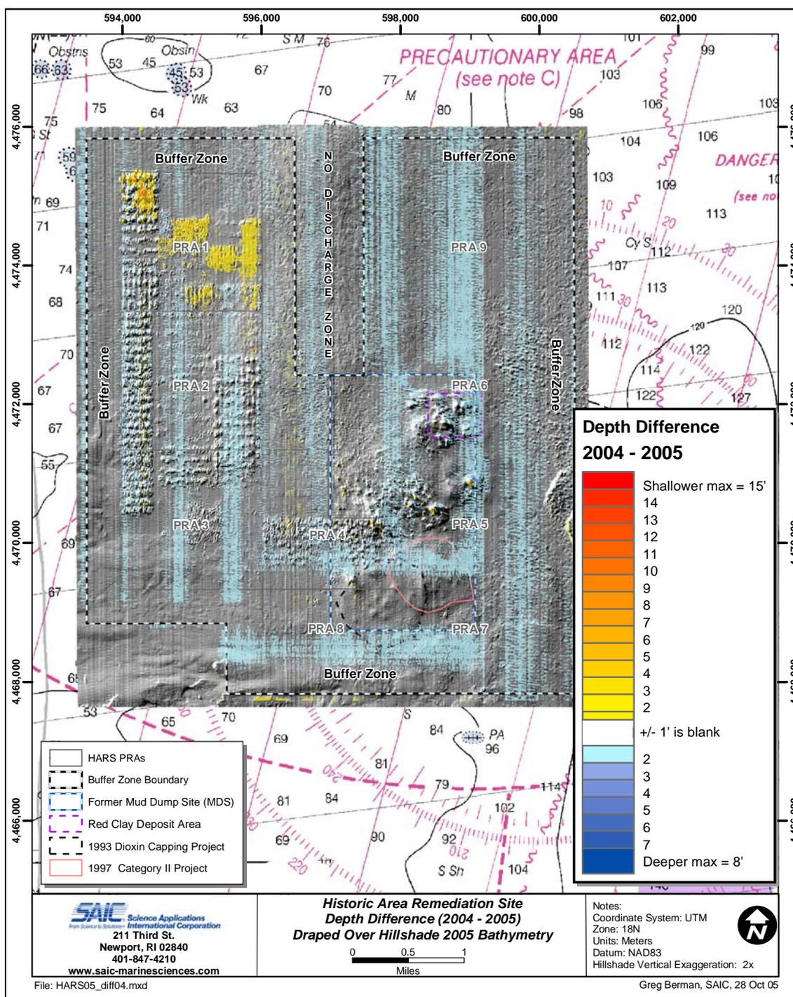
Figure 3.2-7. Bathymetric depth difference between the August 2005 survey and the 2004 multibeam survey
